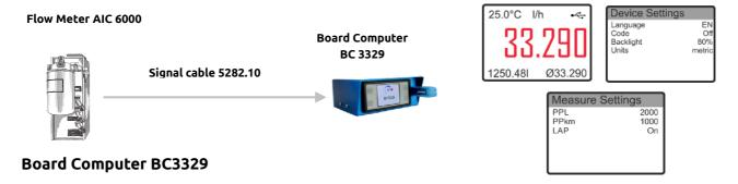
The Board Computer BC3329 Display has input for Flow and Speed sensors. All measured values can be easily seen and written off the large display.
