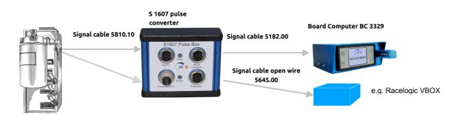
Typical AIC S1607 Pulse Converter Installation with AIC 900, 4000, 800, 1200
